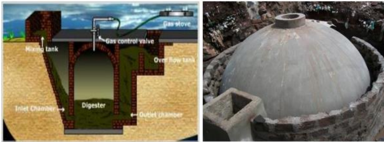
Gambar 9.2. Reaktor biogas tipe kubah tetap ( fixed dome type )
