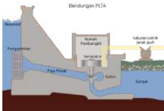
Gambar 2.1: Skema PLTA (Tennessee Valley Authority https://www.eia.gov/energyexplained/hydropower/ )
