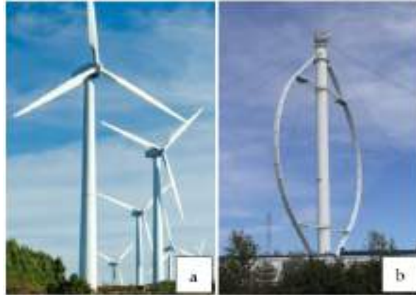
Gambar 3.1: Pembangkit listrik tenaga bayu (a) HAWT- Horizontal Axis Wind Turbines, (b) VAWT-Vertical Axis Wind Turbines
