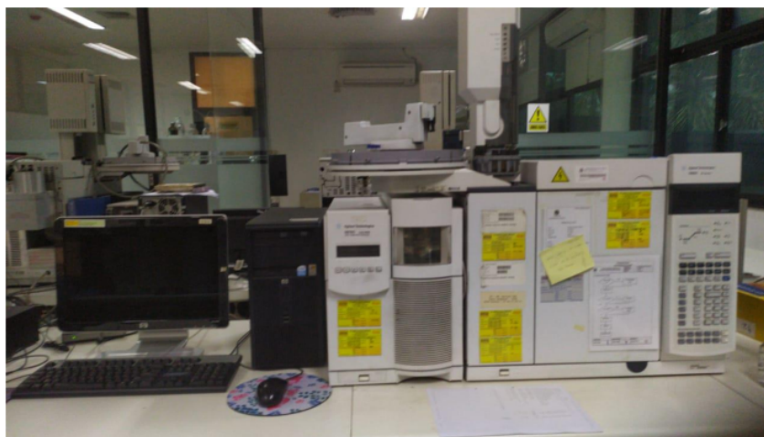
Figure 2. GC-MS equipment for the analysis of citronella oil chemical components
