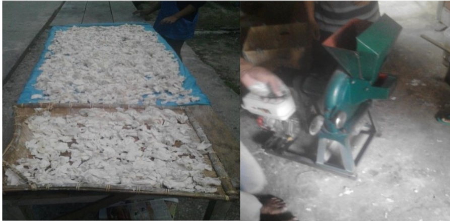
Figure 7. Taro tuber drying process using sunlight and disk mill grinding machine
