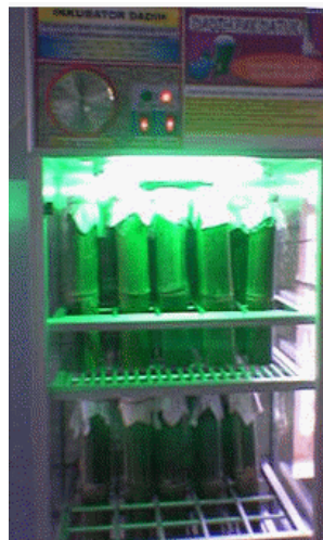
Incubation with Incubator. Specification: Frame: Aluminum Wall: 2mm glass Dimension : 40x40x150cm over: AC 220 60W Control system: Thermohygro regulator Temperature: 39 °C Humidity: 60% RHP
