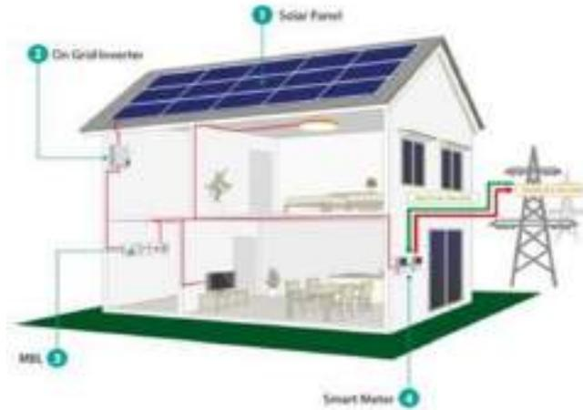
**Gambar 3.6:** PLTS Roof-Mounted atau PLTS Rooftop (Adyasolar, 2018)
