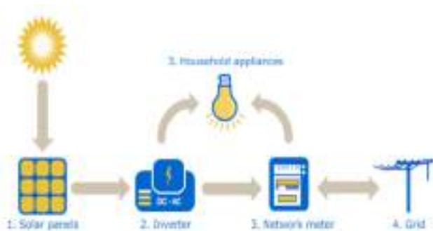
**Gambar 6.4:** Residential grid-tied solar PV system diagram [4]
