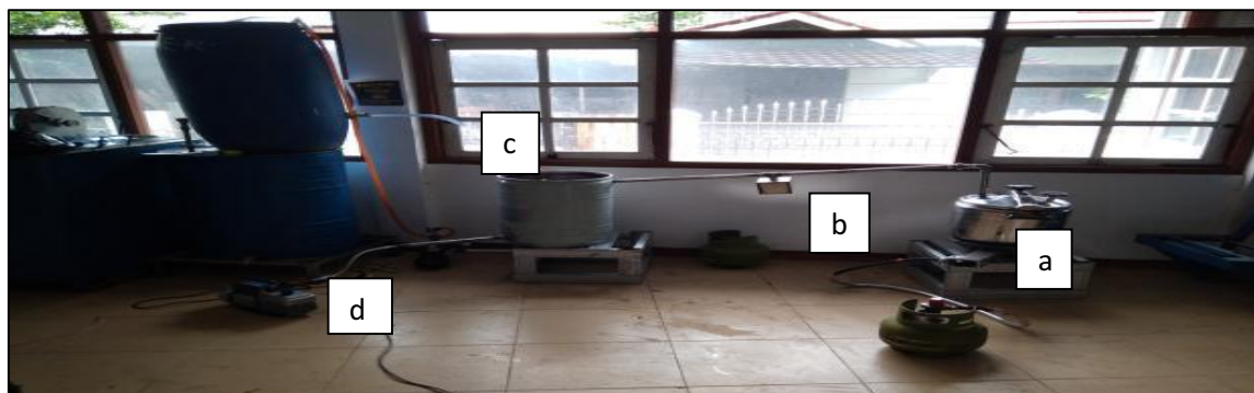
Figure 1. Construction of the liquid smoke maker: a). Pyrolysis tube b). Smoke pipe, c) Condenser, d). Liquid smoke container.
