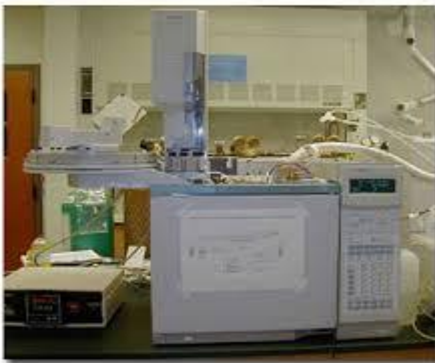
Figure 2. GC-MS instrument for analysis of chemical components of cocoa rind liquid smoke
