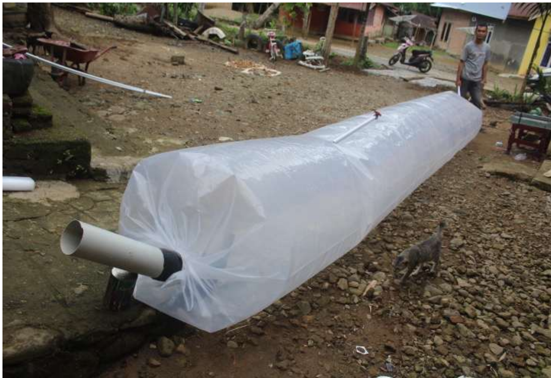
Figure 3. digester balloon type 6 meters long part.
